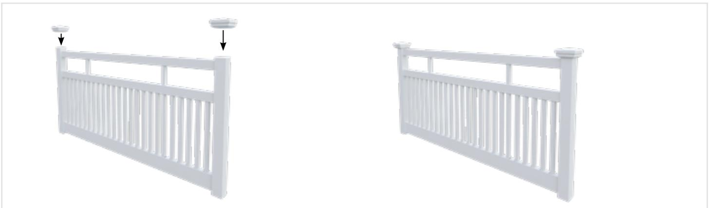
13 Repeat process for remaining posts. Apply silicone to inner of top caps and press on to each post to finish.
