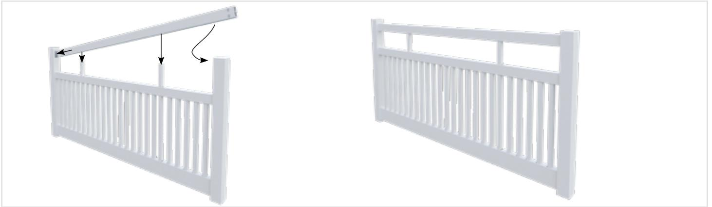
12 Install top rail over long pickets guiding pickets into holes on underside of top rail. Insert top rail into one post and then lever into adjacent post.
