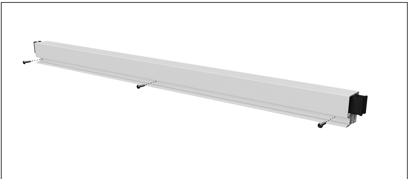
18 Secure with Gate Infill three self-drilling wafer screws within the screw channel.
